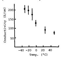
FIGURE 1 Conductivity vs. preparation temperature of polypyrrole.
